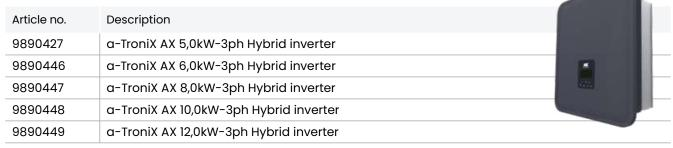
In combination with the single-phase hybrid inverters, one to six AX 2.88 kWh high-voltage battery modules can be operated with an AX 2.88 kWh high-voltage solar storage unit with BMS (5.76 kWh to 20.16 kWh). Together with the three-phase inverters, combinations of two to six battery modules and solar storage with BMS are possible (8.64 kWh to 20.16 kWh).
